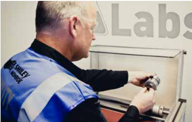
In-house wear resistance (abrasion) testing at Smiley Monroe
