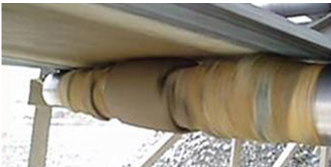
Carryback material buildup on a steel roller
